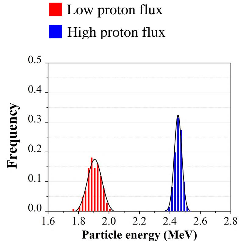
GEANT4 simulation of Bragg peaks and LET profiles in water, simulated energy profiles along the diameter at the air target interface and energy distributions of the high and low flux proton beams at the mylar-water interface. (mean energy = **1.9 MeV – low flux**, **2.45 MeV – high flux**, FWHM = **104.02 keV – low flux**, **56.18 keV – high flux**)
