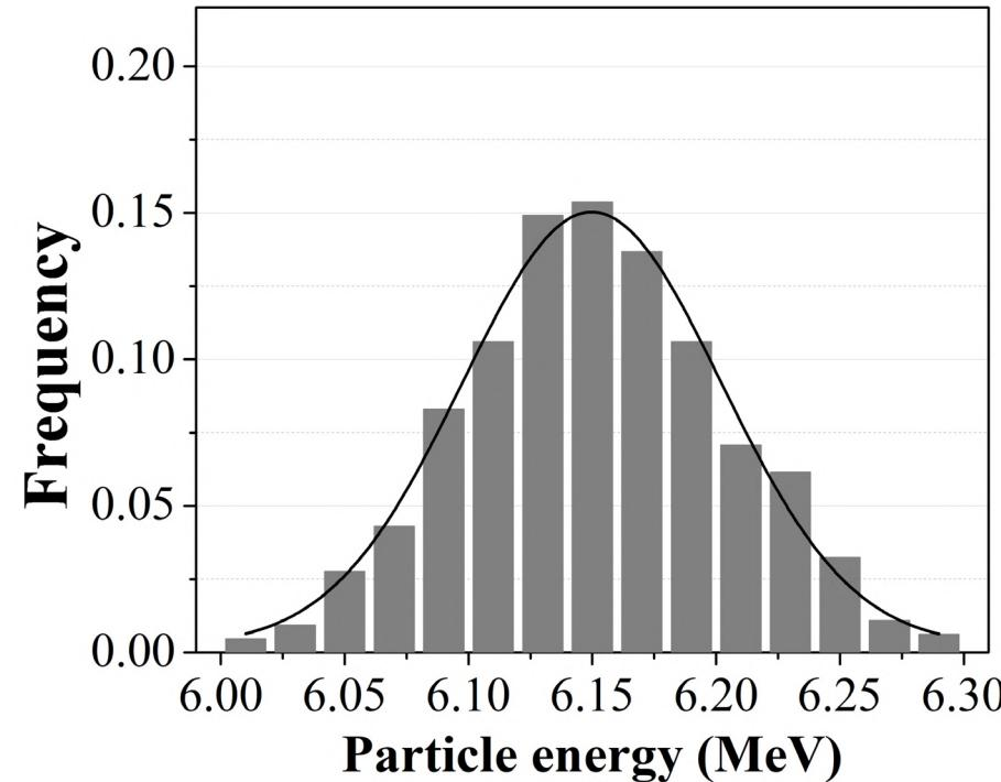
GEANT4 simulation of alpha particles Bragg peak in water against experimental data acquired using the Markus detector and the energy distribution of the alpha particles beam at the mylar-water interface (mean energy = 6.15 MeV, FWHM = 123 keV)
